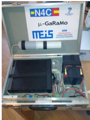
μ-GaRaMo radiological station with SymbioNode node USB-key connectivity
